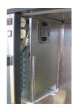
The condensing unit consists of a compressor and a ventilated condenser. The evaporator is located in the internal tank (behind the column) and it has a painting protection in compliance with the regulations in force. The evaporator is also equipped with two fans and a tank for defrosting water collection.
